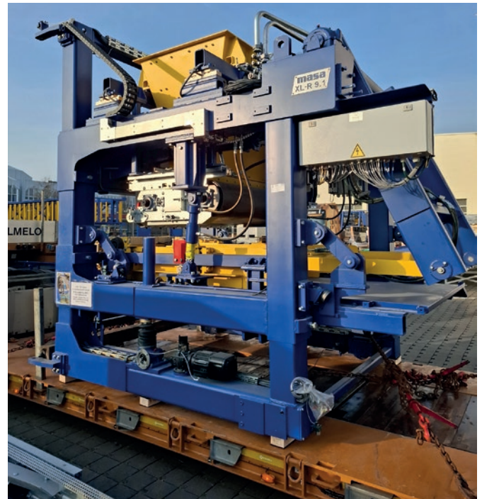
Face mix filling unit of the XL-R 9.1 prepared for transport to Algeria
