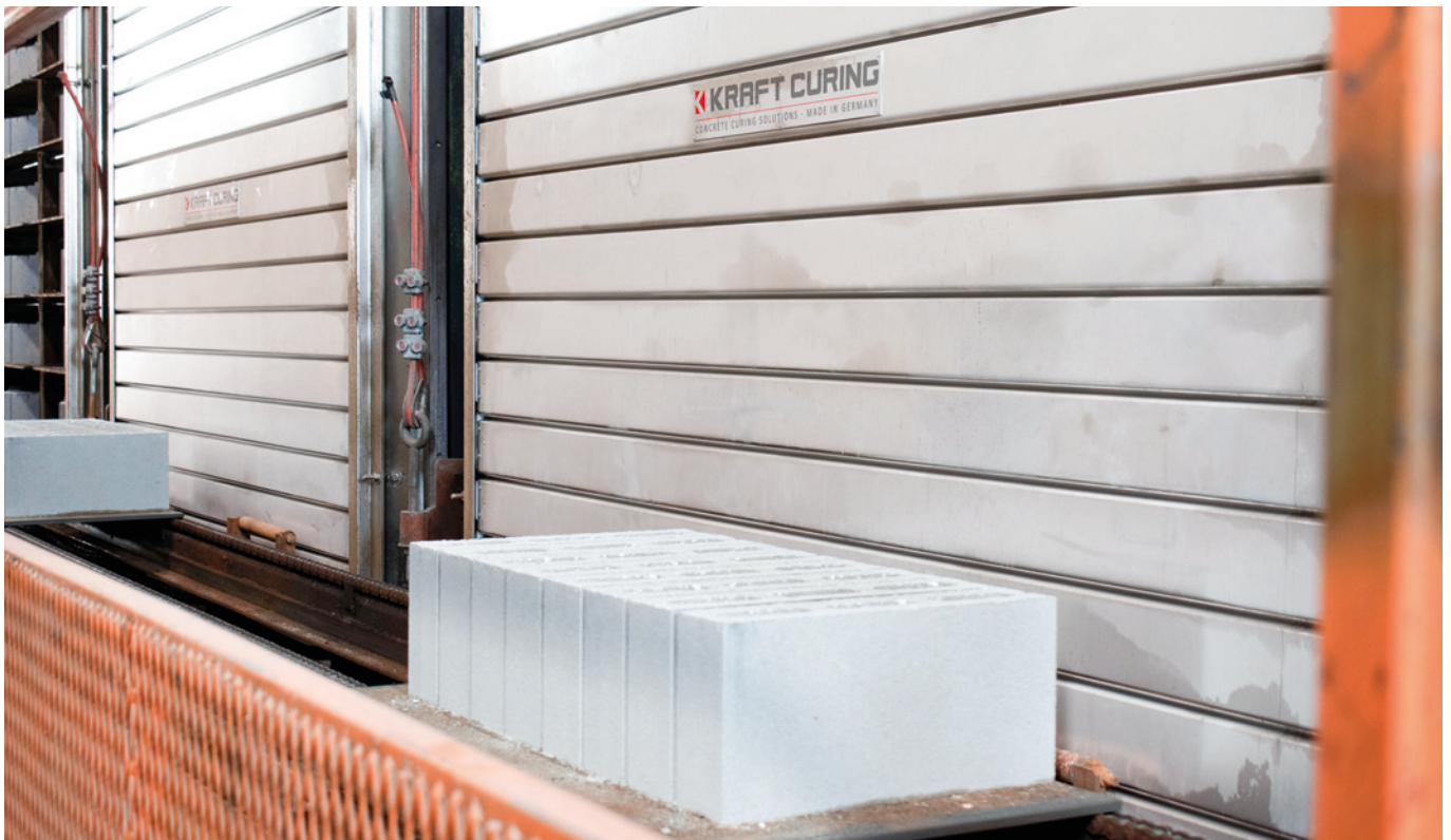
Cured Thin Block moving down the ABC conveyor
