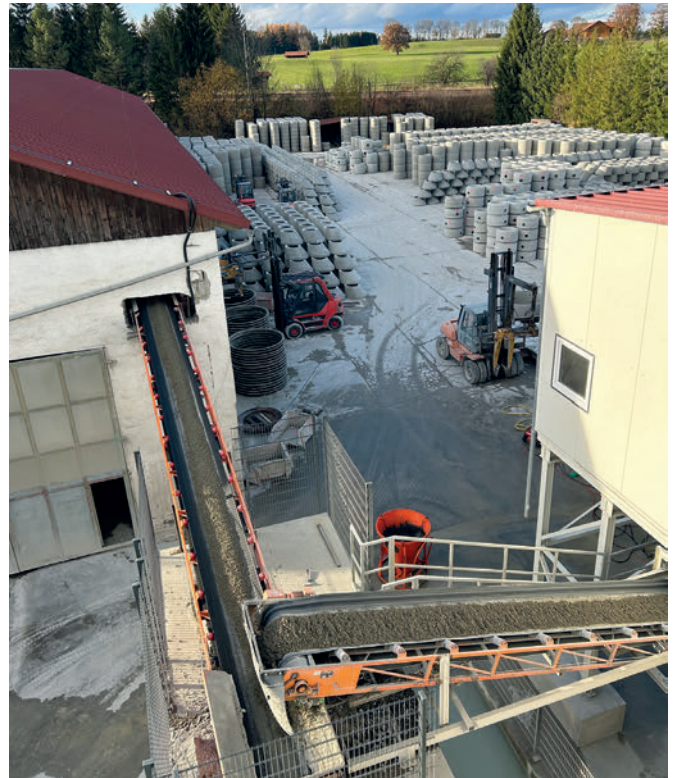
Earth-moist concrete runs directly into the production area via conveyor belts.
