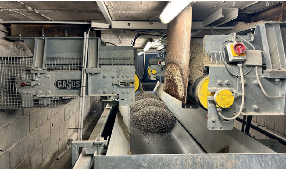
The dosing belts under the individual aggregate silos from the stockpile dose onto the new weighing belt.
