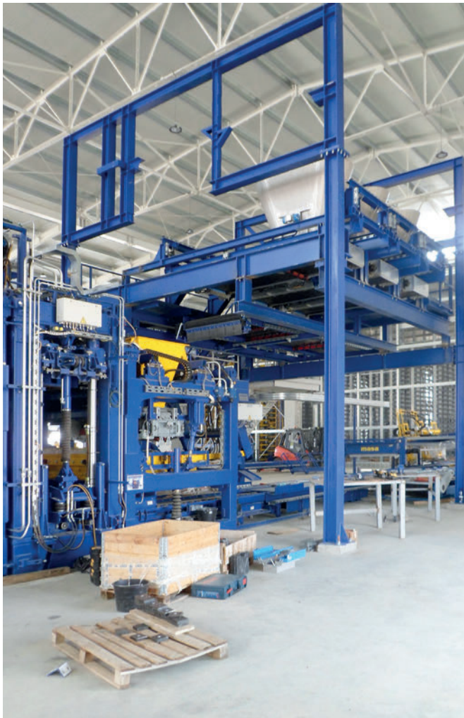
The assembly of the actual heart of the production plant, the Masa XL-R with Multi colour system (here for face mix concrete) required some routine and sensitivity.
