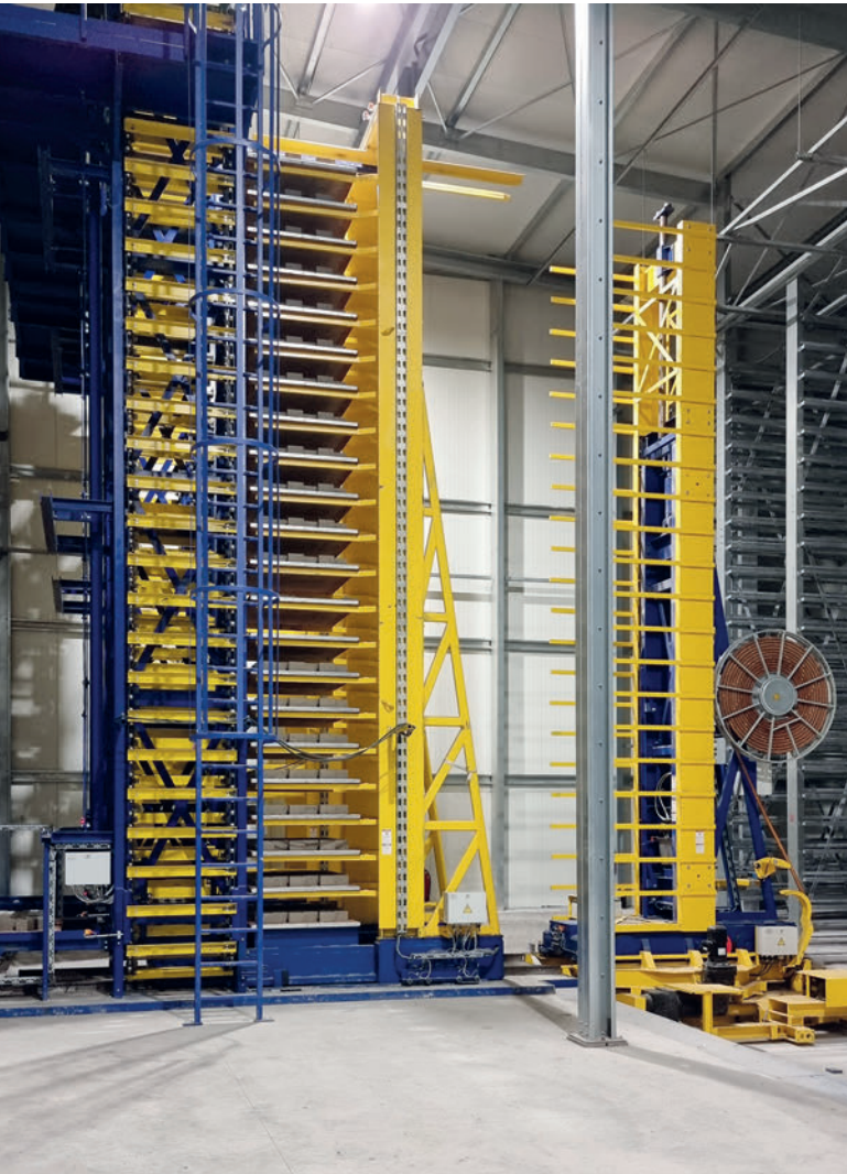
For the transfer of the cured products from the curing area to the return transport, the Masa plant control system coordinates the components finger car, intermediate finger car and lowerator.
