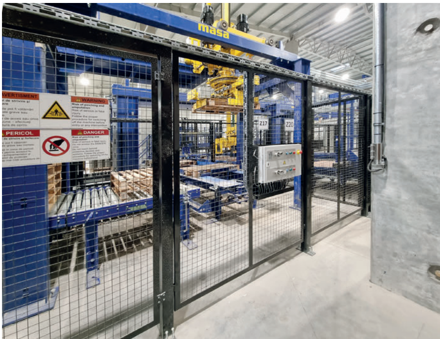
The Masa transport pallet grab precisely feeds the transport pallets to the Cuboter.
