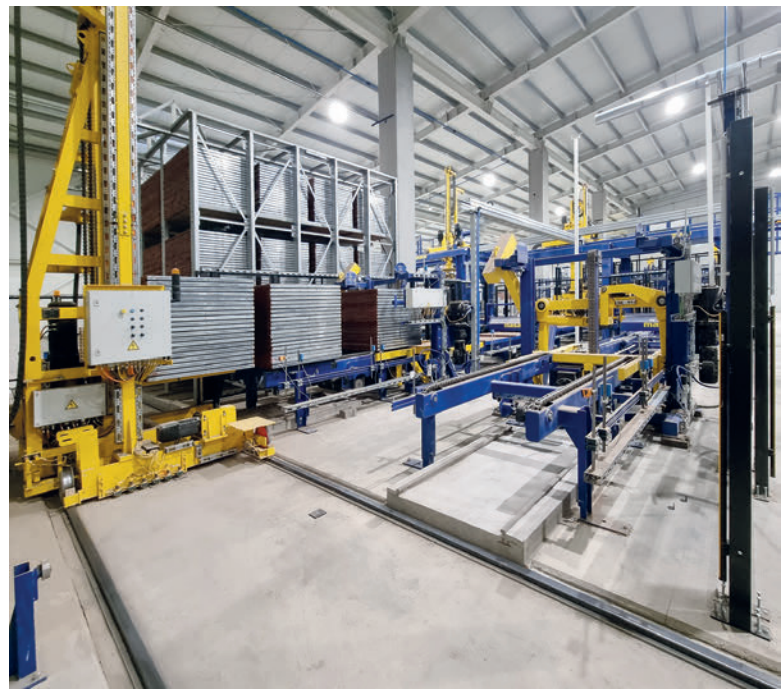
The Masa transport car reliably stores and retrieves the empty production boards in and out of the storage rack.
