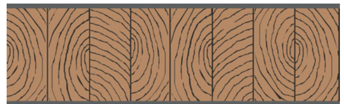
Boards with predominantly vertical annual rings are utilised for enhanced structural properties
