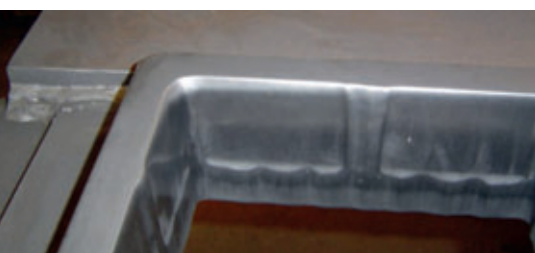
Figure 1: Checking for wear at the lower edge of the mold
