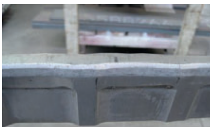
Figure 5: Heavier wear at the upper edge of the mold
