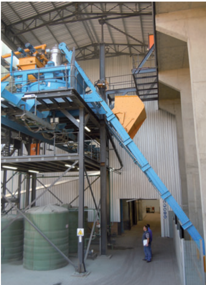
Mixer frame with Masa PH 1500/2250 and PH 200/300 horizontal compulsory mixers
