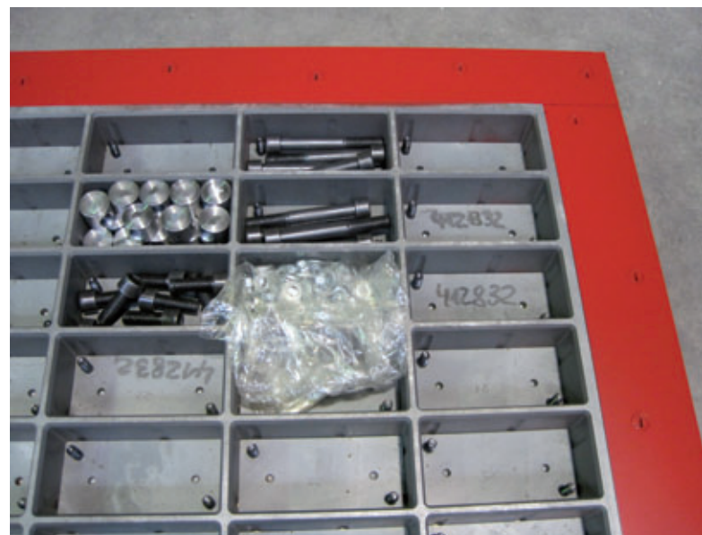
Fig. 2: »Moduline2« mould bottom with separately delivered tamper shoes and mounting kit for bolted flanges
