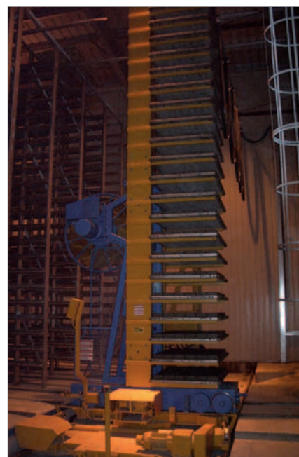
The fully automatic, rotating moving platform loads and unloads the HS shelving installation, which was designed as a closed system with recirculating air equipment.
