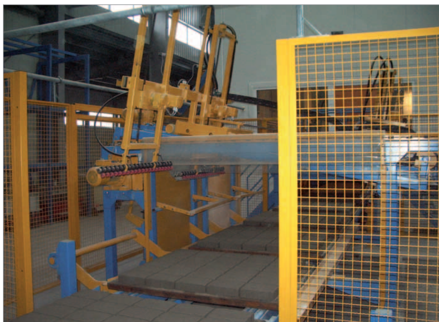
The concrete blocks produced by the machine are transported to the lifting rack by means of a lowering device and a free lift conveyor.
