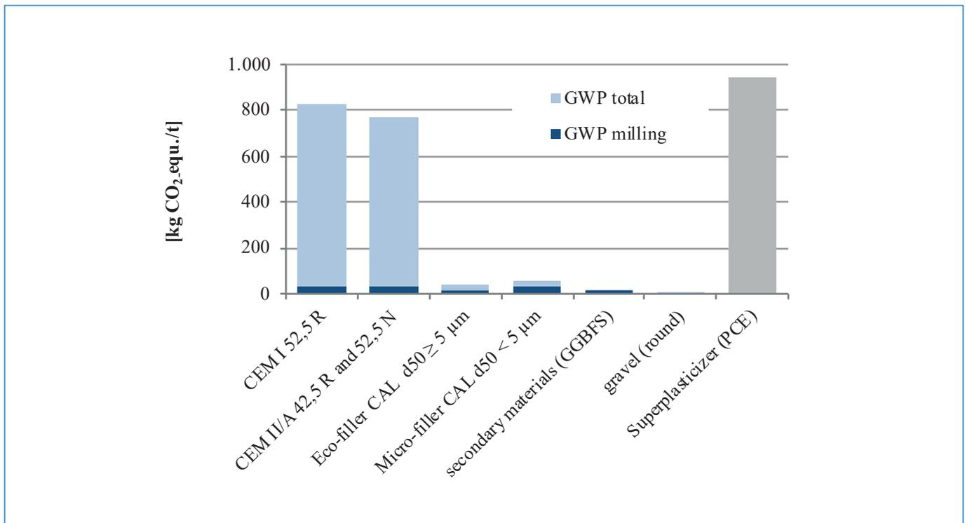
Fig. 2: Total GWP of potential source materials for concrete and the proportion arising from their grinding and screening
