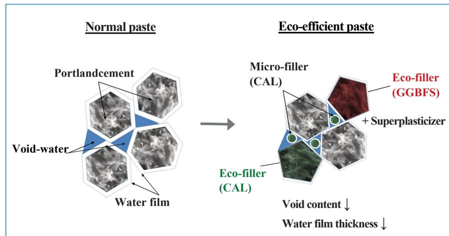
Fig. 1: Packing density optimisation and reduction of water requirements through the combined substances of a fines paste
