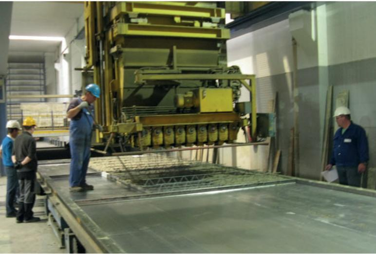
Fig. 4: Producing an outer wall element from eco-concrete
