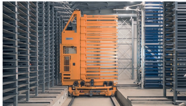
Unlike conventional racks, the Kraft Rack System is an integral part of the curing process itself.
