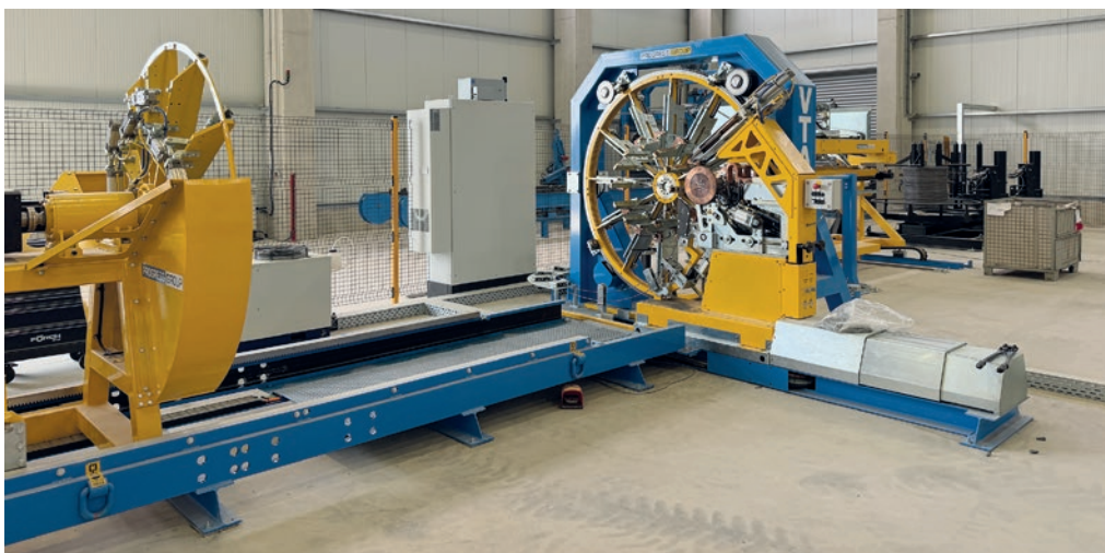
Progress cage welding machine of the VTA series for the production of reinforcement cages.
