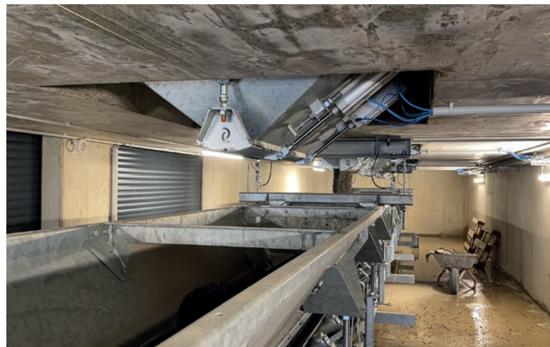
The aggregates are batched via double dosing gates that are integrated into the bottom part of the aggregate bins.
