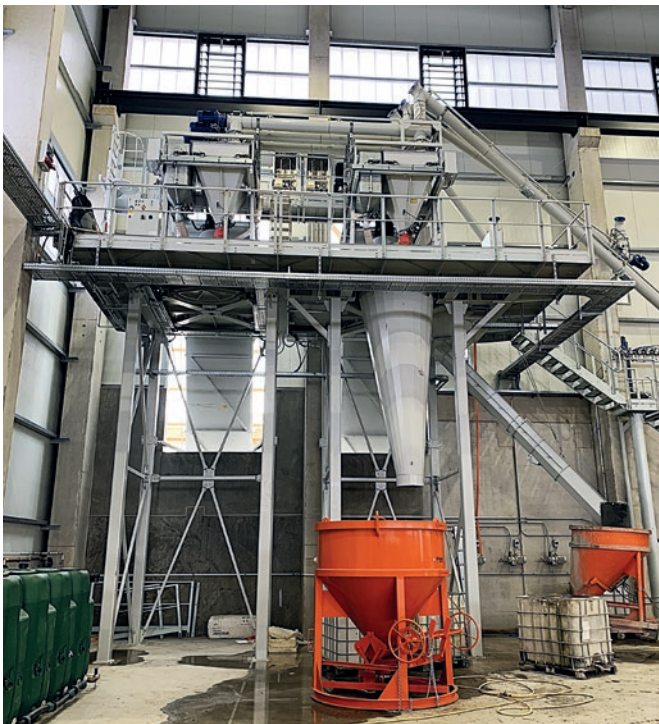
Wiggert's twin mixer plant was delivered in factory-prefabricated modules, enabling fast and easy installation.
