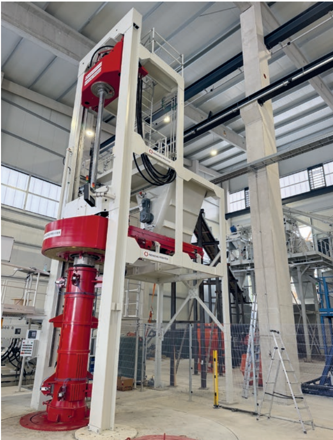
Radial press RP from Prinzing Pfeiffer, a high-performance machine for the production of pipes made from conventional concrete and reinforced concrete as well as for pressure pipes in various sizes, and the first reinforced concrete pipes produced in Nisterau.
