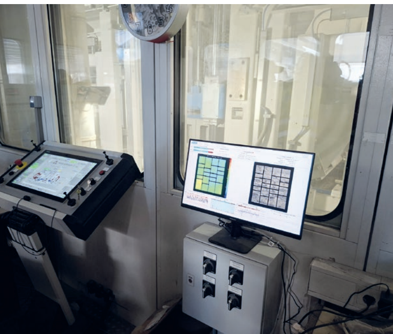
Visualization of quality control at the control console of the concrete block machine Multimat RH 1500-4
