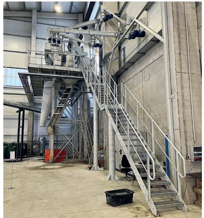
Wiggert's twin mixer plant was delivered in factory-prefabricated modules, enabling fast and easy installation.
