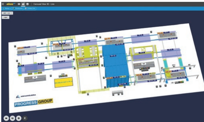
Full transparency with the GPA (Graphical Performance Analyzer) in ebos rc through 3D visualisation of the circulation plant.
