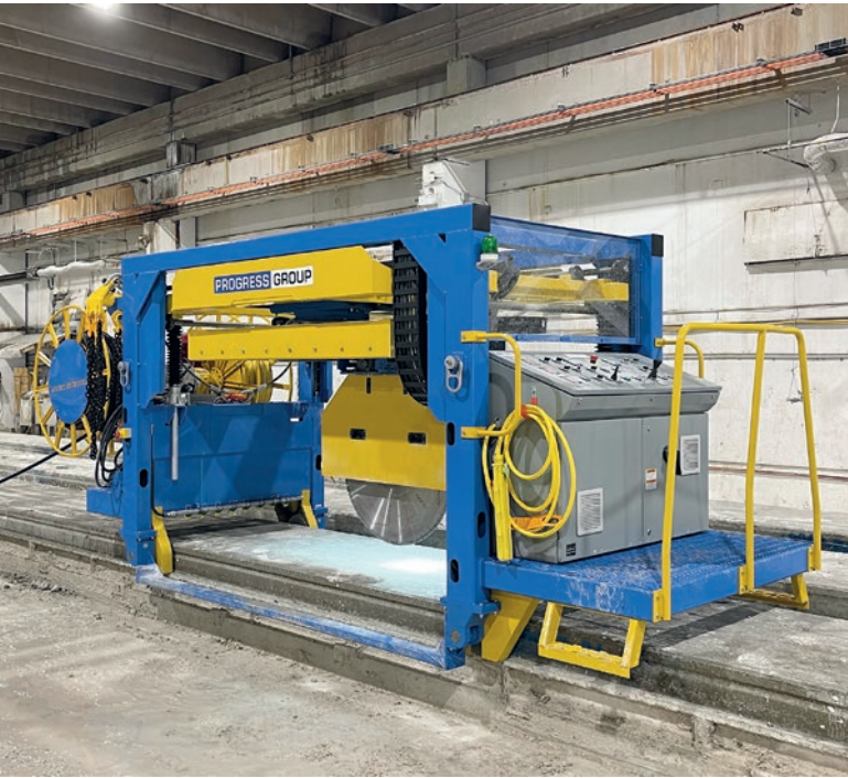
The Angle Pro saw cuts concrete at any angle.
