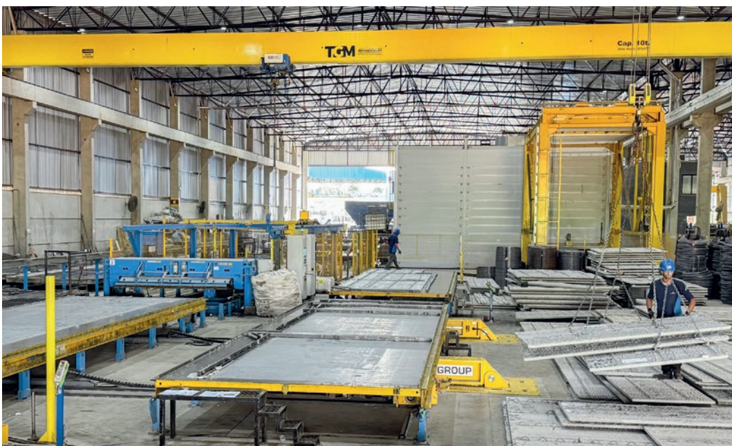
A view inside the new plant of the Brazilian precast manufacturer – up to 1,200 m 2 of precast slabs with in-situ topping and double walls are produced here per shift.
