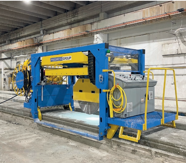
The Angle Pro saw cuts concrete at any angle.
