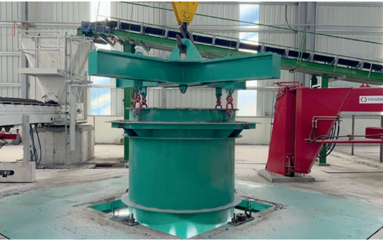
Lifting process with overhead crane
