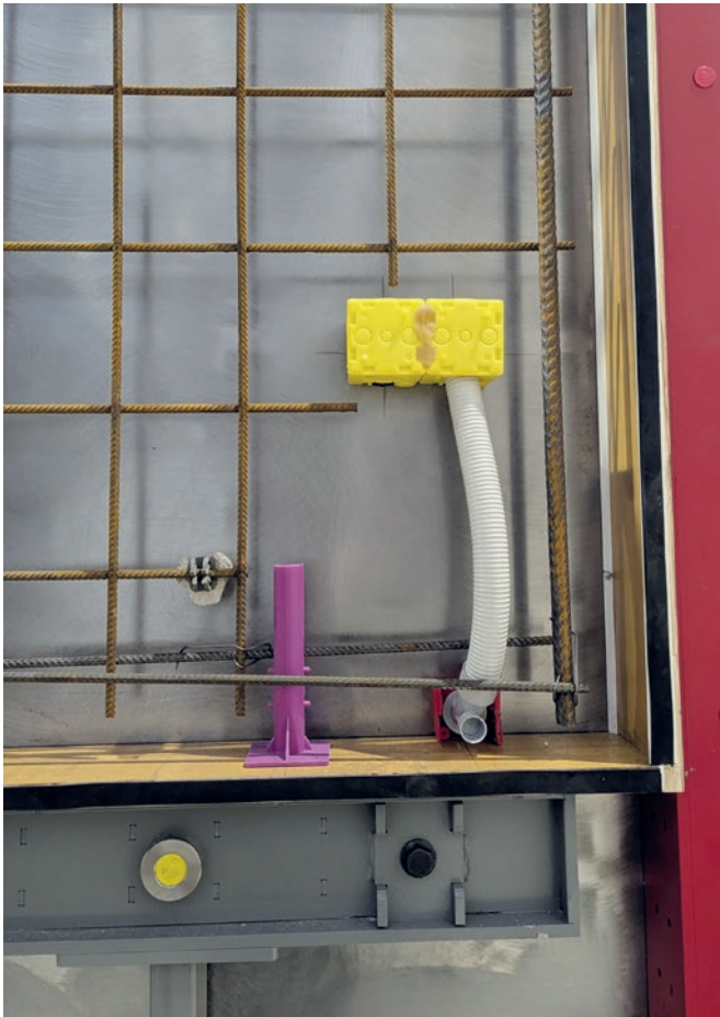
The magnet-based base and side formers are designed for wall thicknesses of 100 to 250 mm
