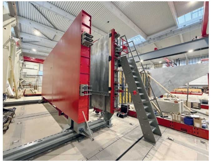
Compact single-cavity battery mould with an option for future expansion
