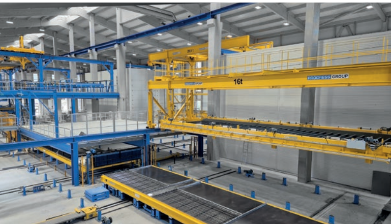
The automatic turning device is used in the production of double walls.
