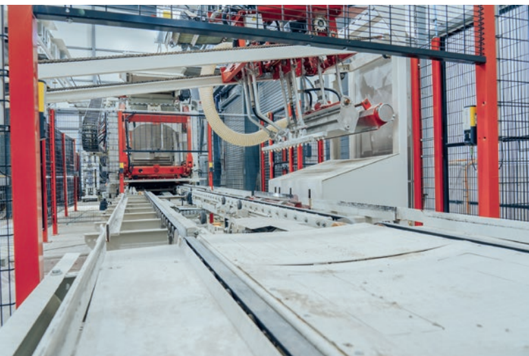
On the wet side, products pass through the washing unit.
