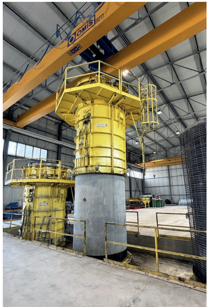
Demoulding the outer mould—another pipe is ready for retrieval
