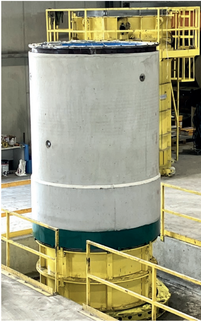
Recently demoulded interjack pipe with partially reduced wall thickness
