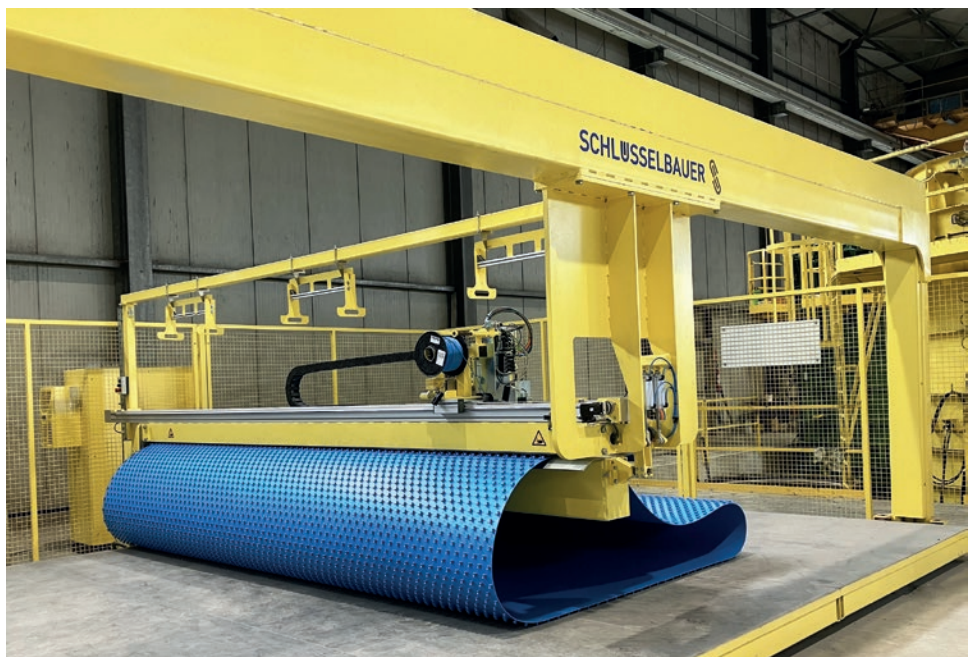
The plant for automatic welding of Ultra-Grip PE concrete protective liners into cylinders—a key step in the production chain at ILCEV
