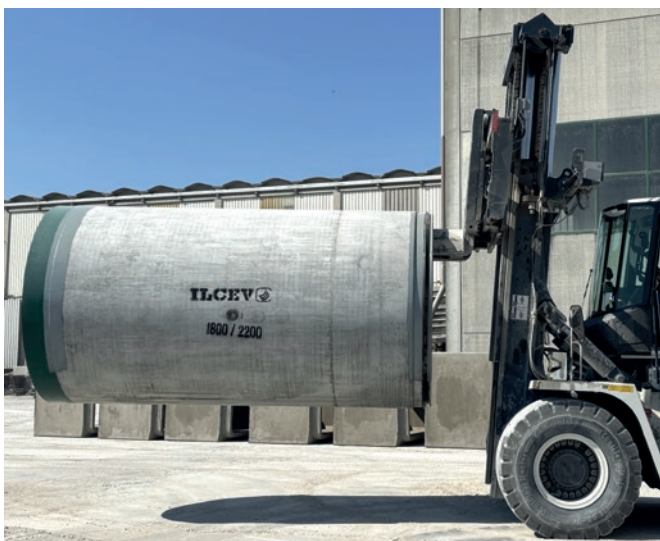
Gentle loading of PE-lined pipes using jacketed forklift tines ILCEV specializes in the manufacture of pipelines for pipe jacking. Since 2024, it has been part of the Gruppo Grigolin, an international group of companies focusing on the construction and engineering industry.
