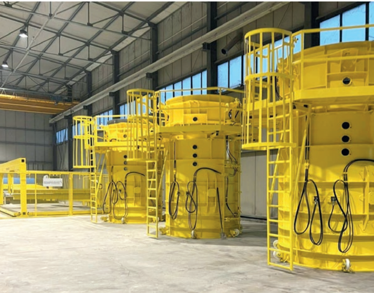
Schlüsselbauer Technology plant for liner processing and pipe wetcast moulds before final start-up
