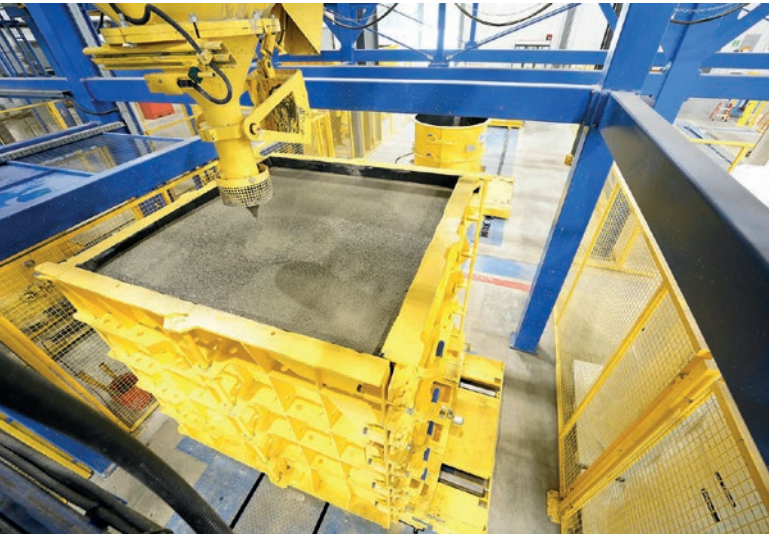
Perfect Forming Technology—square in this case—designed for processing SCC; all sealing elements are machined to high precision at Schlüsselbauer Technology
