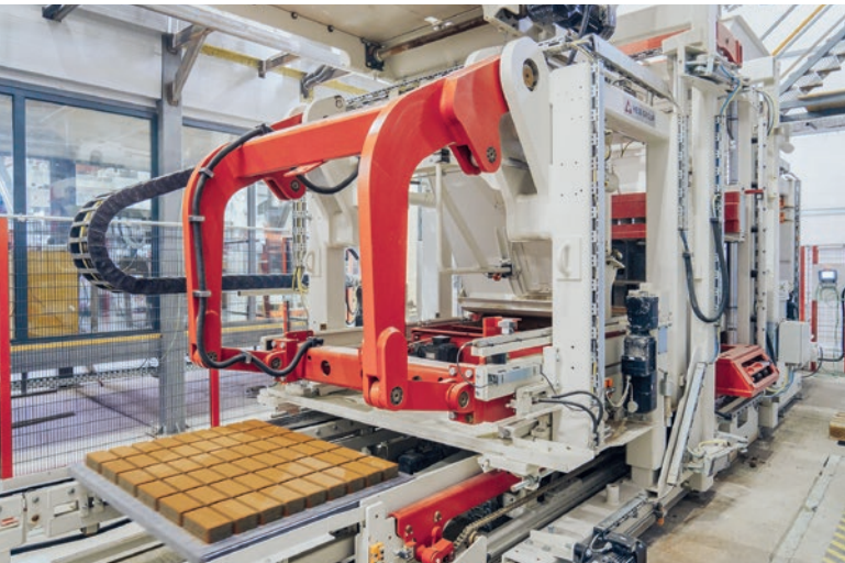
The RH 1500-4 MVA forms the technological heart of block and paver production
