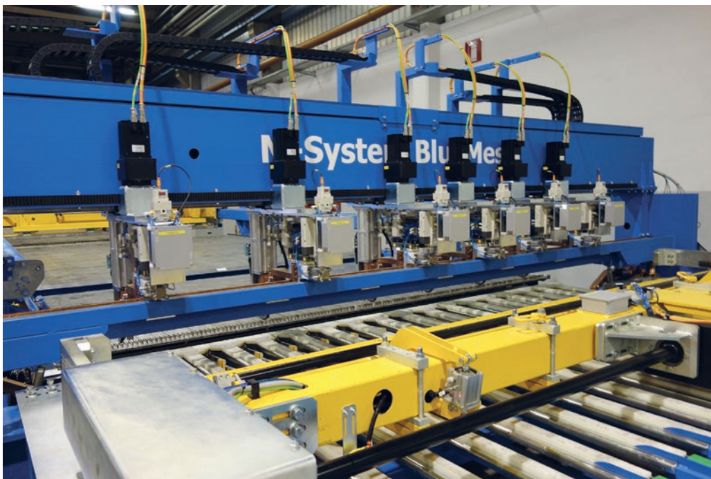
The M-System Blue-Mesh® mesh welding plant produces bespoke mesh from coil according to individual specifications.
