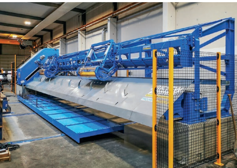
The MSR 20 straightening, cutting and bending machine is designed for the production of tailor made reinforcement bars.
