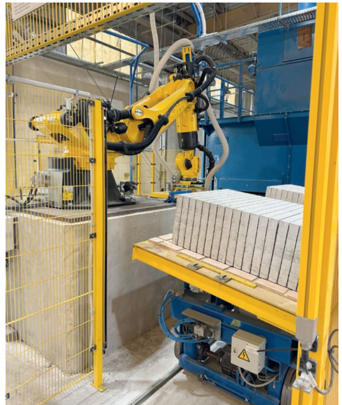
Transfer carriage system with robot loading system
