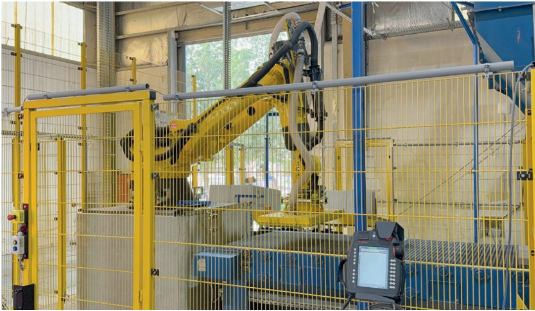
Loader robot placing products onto the shotblasting conveyor belt
