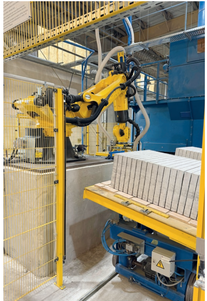
Transfer carriage system with robot loading system
