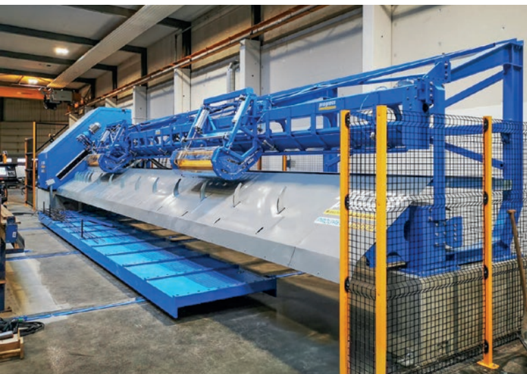
The MSR 20 straightening, cutting and bending machine is designed for the production of tailor made reinforcement bars.
