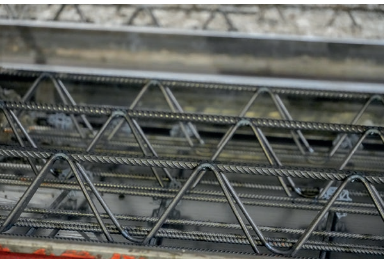
The special feature of the machine: Lattice girders with different wire diameters for the top and bottom chords.
