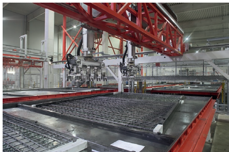
The lattice girders and reinforcing bars are placed precisely on the pallets using the grippers.
