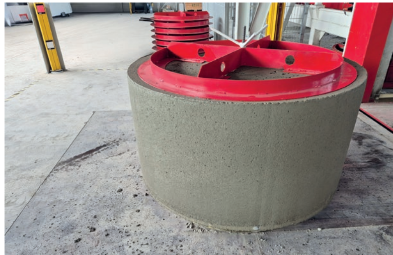
Manhole base DN 1000 (42") with support element for curing, also manufactured on the Tornado 150/150
