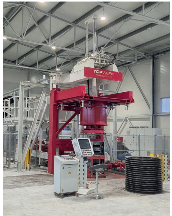
Tornado 150/150: Automatic underfloor vibration machine for the production of manhole components and related precast concrete elements
