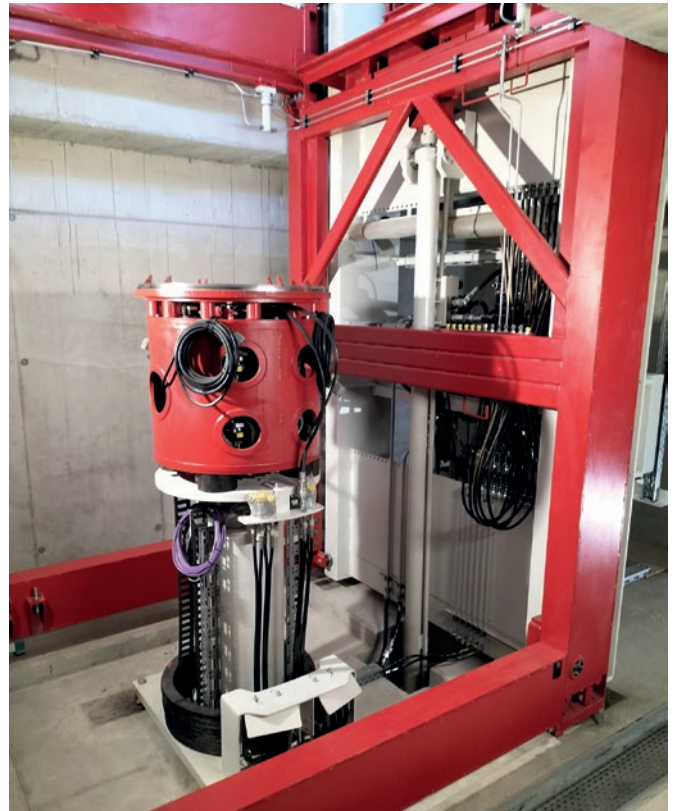
Vertical compactor VTA 150 with amplitude control and lifting device
