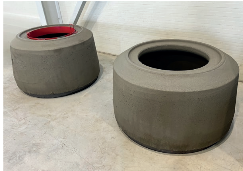
Manhole cone DN 1000/625 height: 600 mm with offset entry, manufactured fully automatically on the Tornado 150/150
