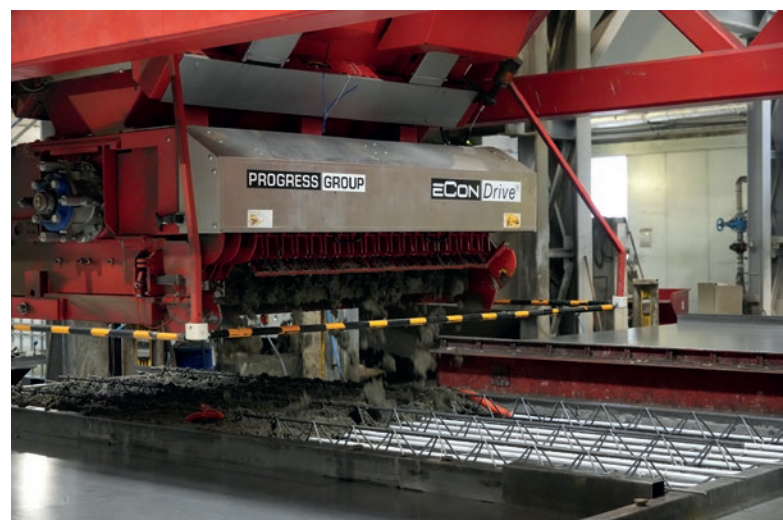
The concrete spreader ensures even and precise discharge into the shuttered pallets on the production line.
