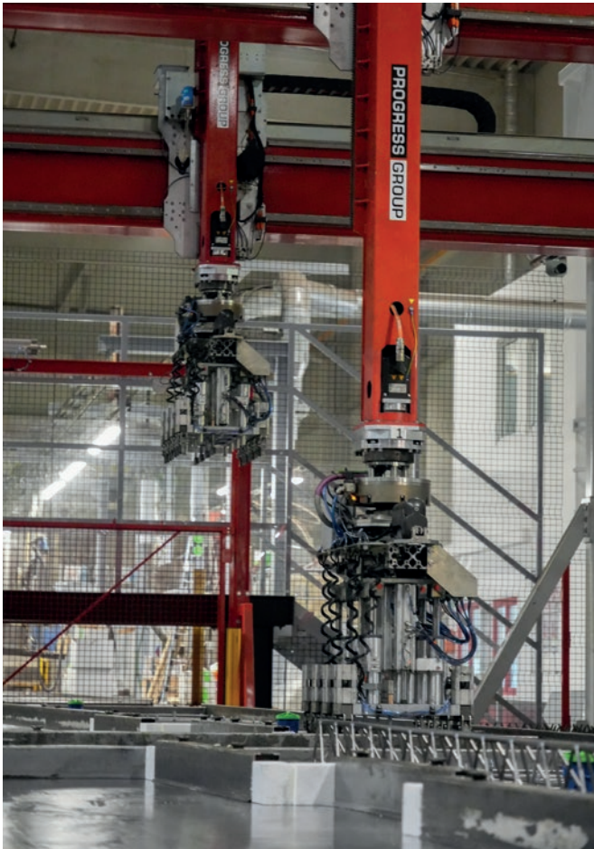
In the Wire Centre, reinforcing steel is processed and laid fully automatically from the coil.
