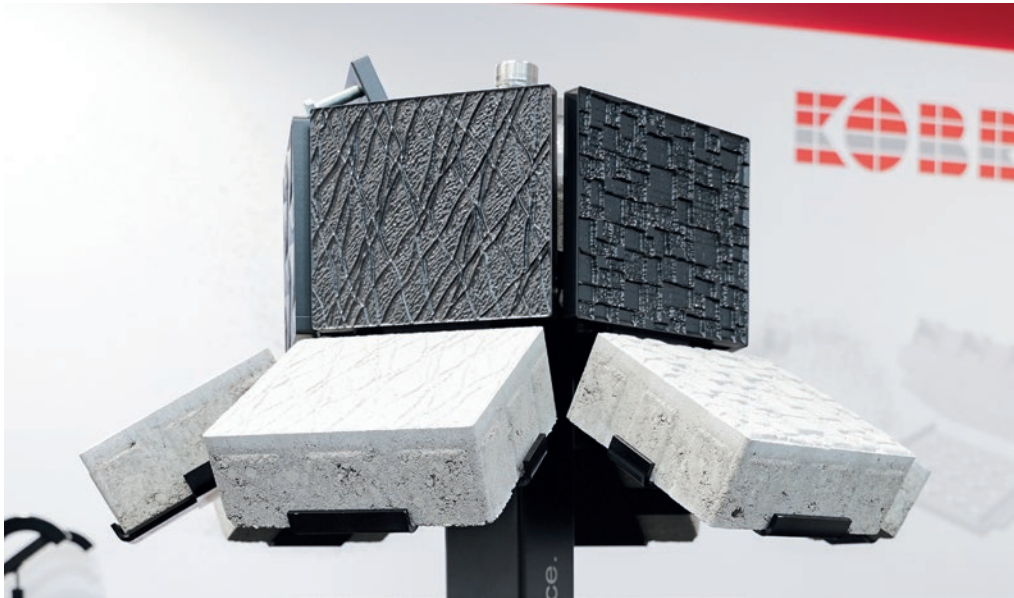
Exhibit at bauma 2025 - AM-manufactured tam- per shoes and pavers produced with them
