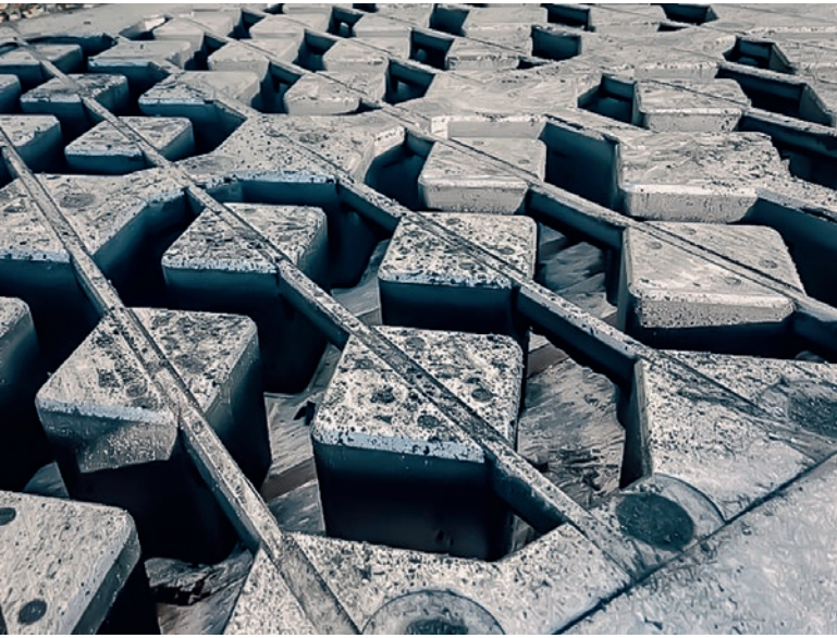
Printed cores without weld seam in mold insert
