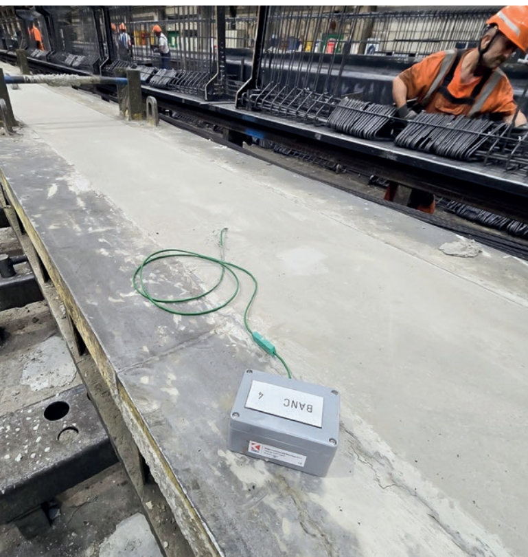
A heavy-duty magnetic wireless temperature transmitter (gray enclosure) with Type K thermocouple wire for internal concrete temperature measurement
