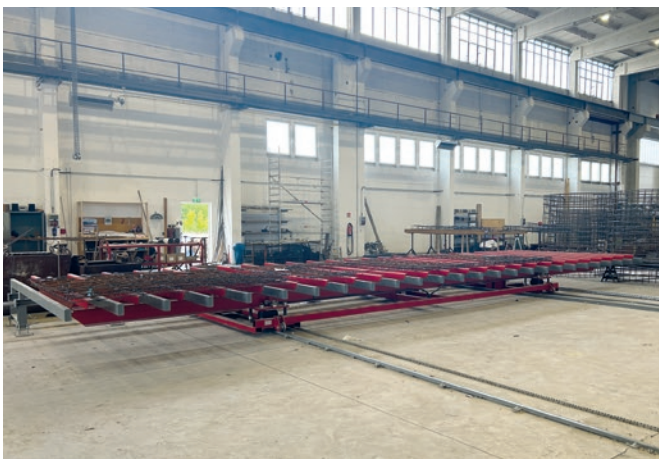
Special transfer carriage for transporting the reinforcement to the circulation plant
