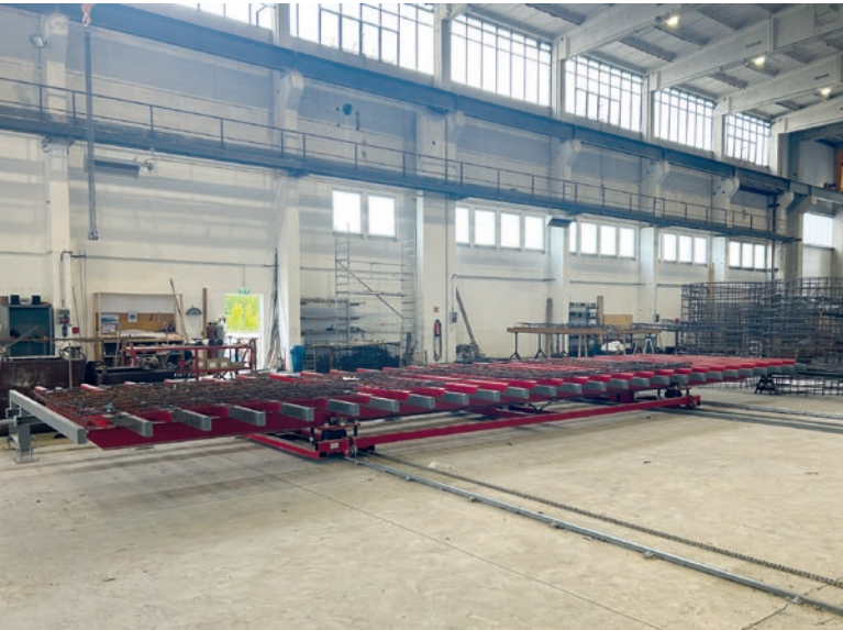
Special transfer carriage for transporting the reinforcement to the circulation plant
