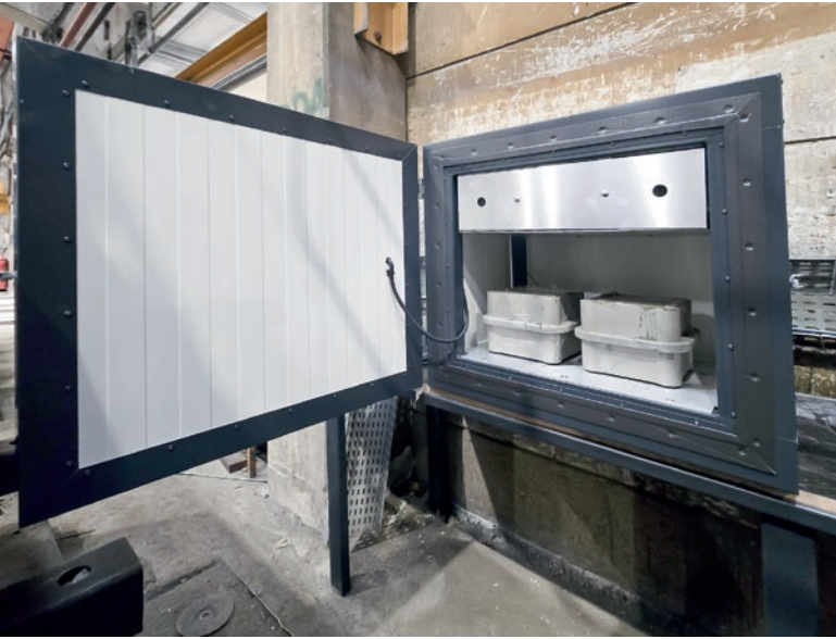
Insulated Match-Cure environmental chamber with test specimen with internal concrete temperature measurement.
