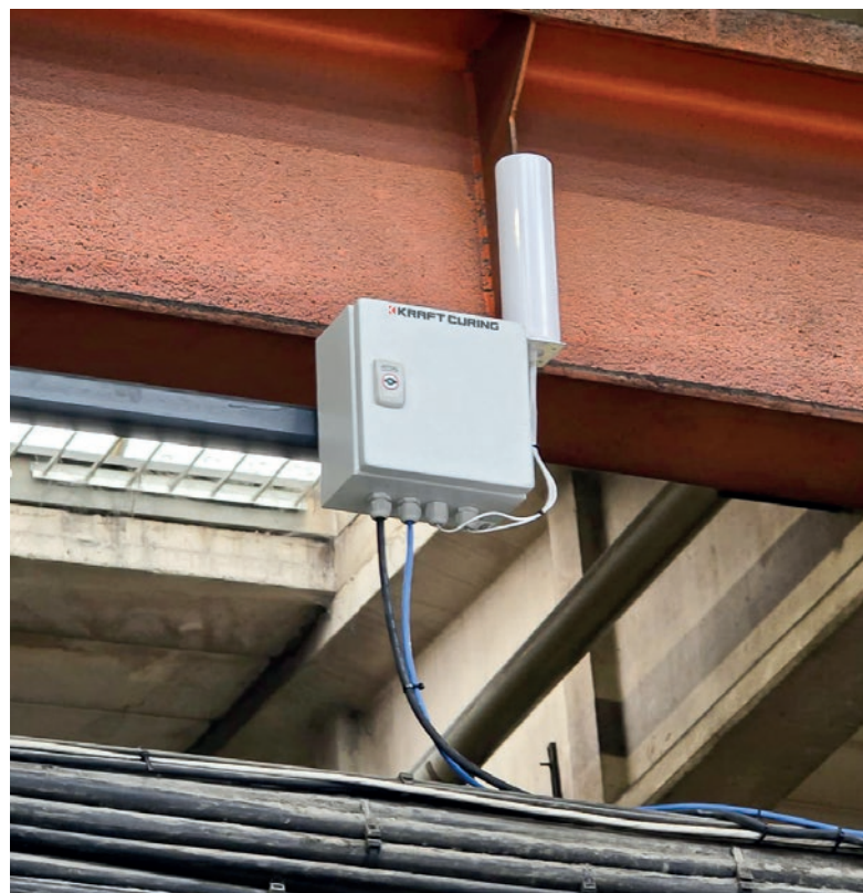
A wireless repeater placed throughout a factory or yard to ensure excellent signal strength throughout a large area. thermocouple wire for internal concrete temperature measurement
