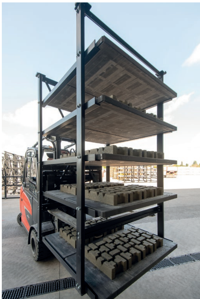
Five-level racks loaded with freshly produced concrete blocks ready for curing.
