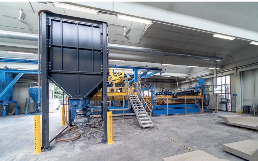
The 3D concrete printer sets new dimensions in precast construction.
