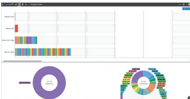
The WorkloadProfiler in profit YC provides an overview of the current utilisation of machines. Through machine learning, the duration of production jobs can be predicted.
