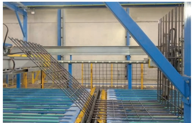
Two separate bending systems enable the production of huge reinforcement cages for heavy precast elements.
