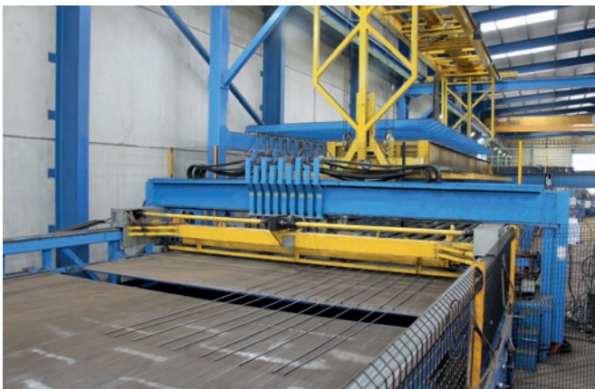
The M-System Evolution mesh welding plant in Byley boosts operational efficiency.
