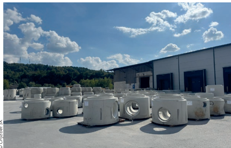
The made-to-order monolithic manhole bases at the warehouse
