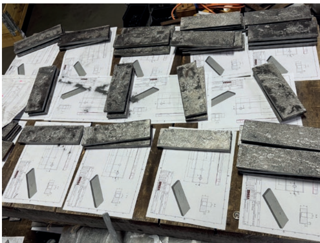
Tamper shoes with embossed surfaces from the 3D printer
