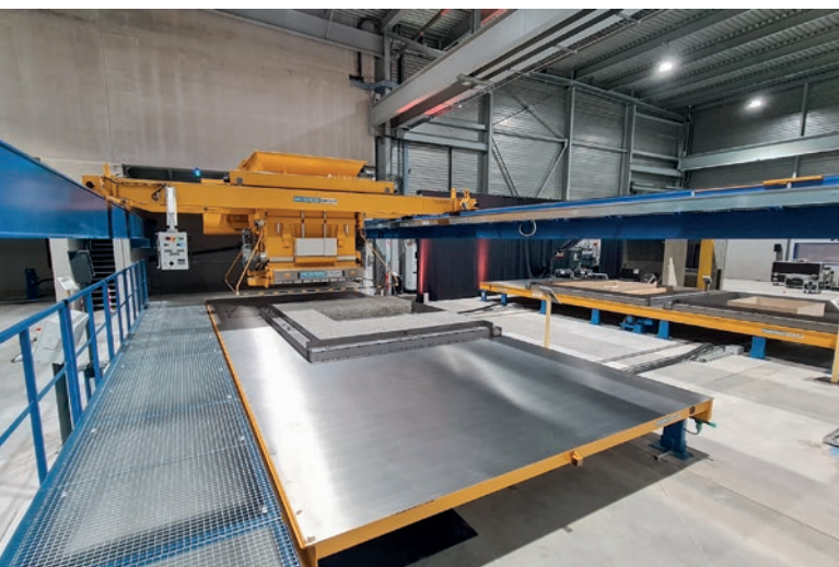
The newly designed concrete spreader is used to discharge the wood-concrete.
