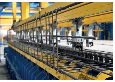
The integrated beam bending system guarantees an efficient production of reinforcement cages.
