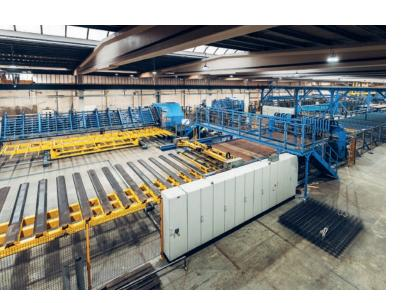
The M-System PowerMesh welding plant is producing a high output of customized mesh with flexible spacing and bendings, increasing both speed and volume capacity.
