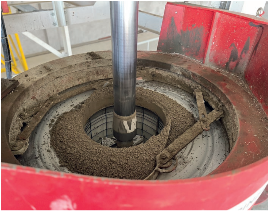
Concrete pipe production with the worldwide proven radial pressing process
