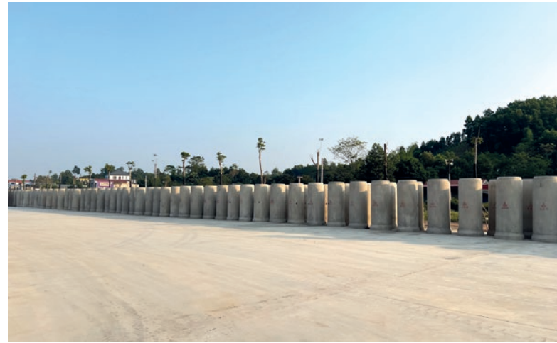
Storage area for cured concrete pipes. Produced with the radial pressing method
