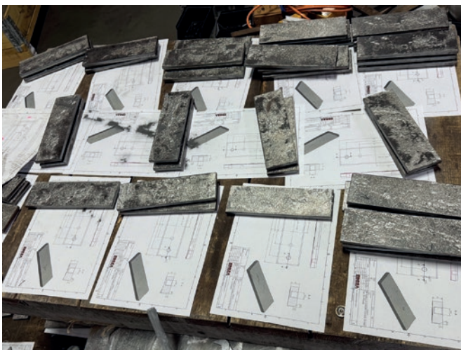
Tamper shoes with embossed surfaces from the 3D printer
