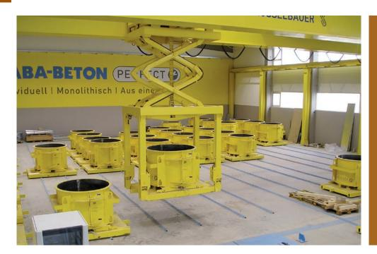
One of the first largely automated Perfect Base production plants installed at HABA Beton, one of Europe's leading providers of concrete pipes and man-
