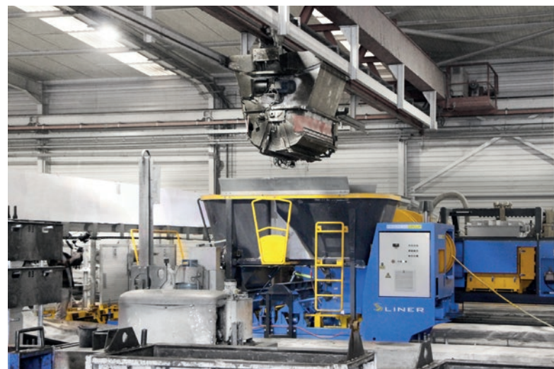
The S-Liner® slipformer ensures automatic production of prestressed concrete slabs with less cement.
