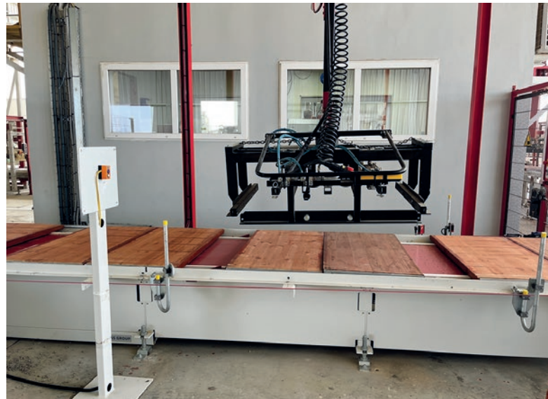
Manually operated, pneumatically working 4-side clamp ATZ-P4
