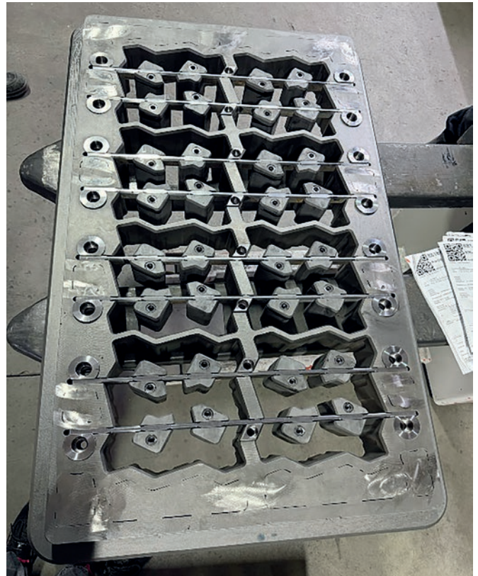
Mold for grass pavers with cores made from recycled material
